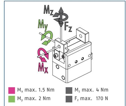
① The indicated moments and forces are static values, apply for each base jaw and should not appear simultaneously. Loads may additionally occur to the moment produced by the gripping force itself.
