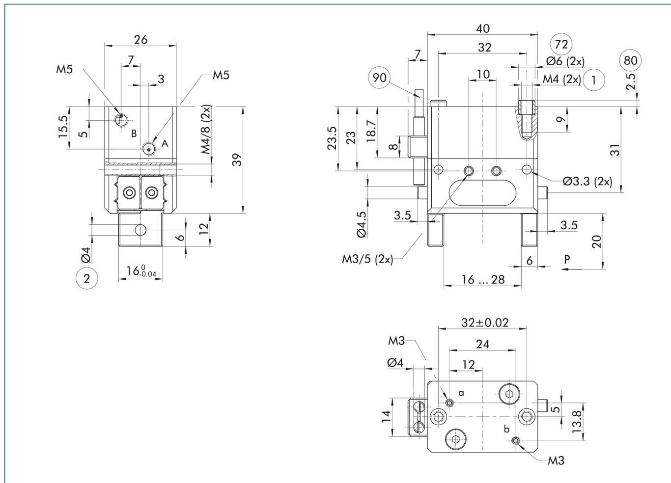
The drawing shows the basic version of the gripper with open jaws, without dimensional consideration of the options described below.
